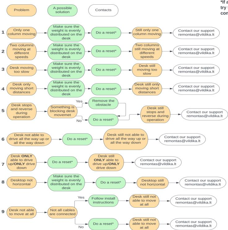
\*If after the reset, the fault has not disappeared try to repeat reset 1 3 more times and only then contact our support
